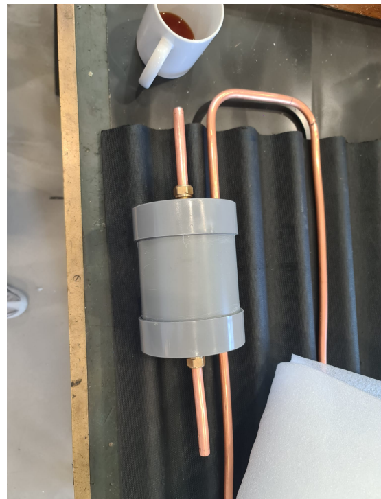
(d) Finished storage vessel without insulation
