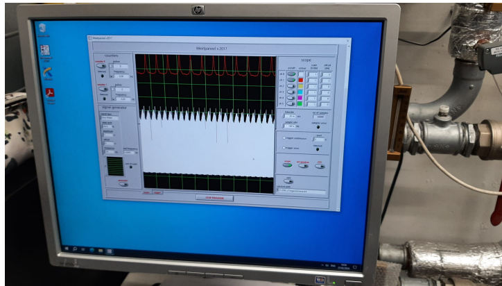
Figure A.3: Experiment 2: Meetpaneel, used to obtain and save the pulse sensor and pressure sensor data.
